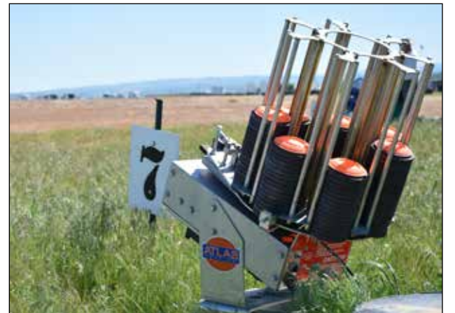
Up close and personal with a clay pigeon thrower. This device rotates through stacks of clays, launching them far and high across the gunner's "shooting lane."
