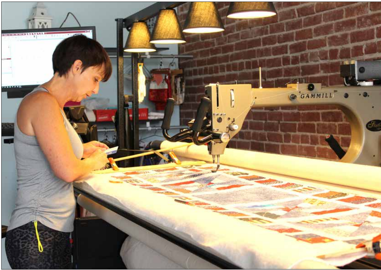
Photo by Michele Smith Vonda Anderson is shown at work on a table runner for her mother, Sherry LaMore. LaMore wanted more “density” in the quilt, so Anderson programmed the Gammill longarm quilting machine to apply feather stitching to it.
