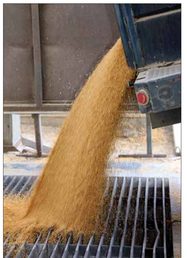
One of Prescott's two ground pile storage units. Grain is emptied into the pit from a truck, taken to the top by the leg system, the same as other elevators. When the pile is complete it is covered by tarps.
