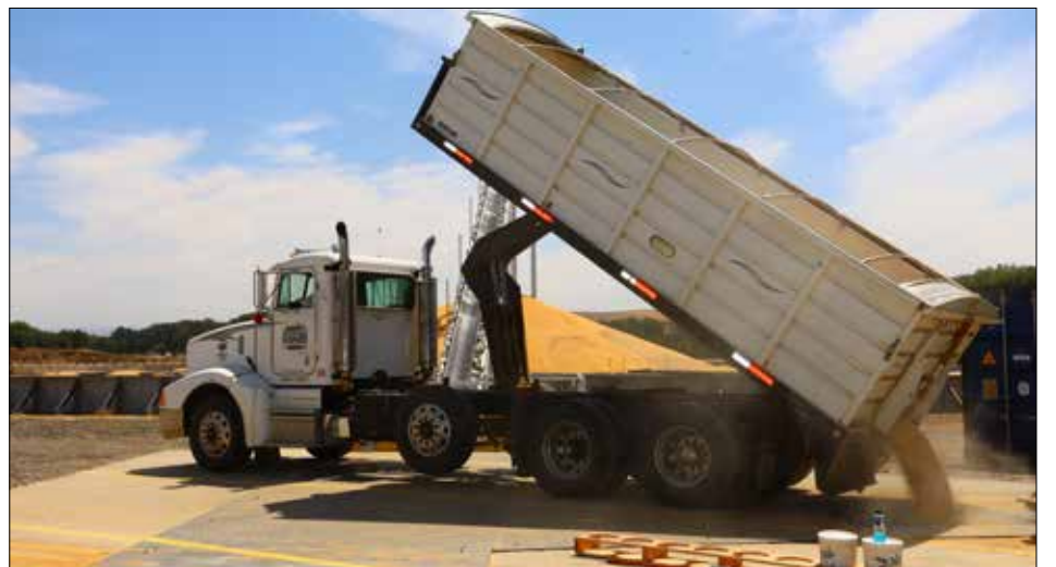
One of Prescott's two ground pile storage units. Grain is emptied into the pit from a truck, taken to the top by the leg system, the same as other elevators. When the pile is complete it is covered by tarps.
