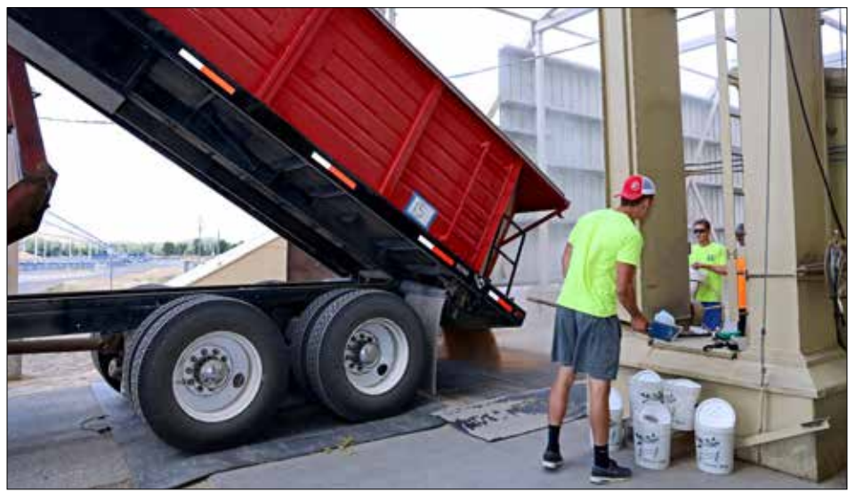
Clockwise from top: An example of a flat house storage unit at Northwest Grain Growers in Prescott. The interior of the flat house showing the first pile of soft white wheat accumulating in the back. The grain is unloaded into an under ground pit where the leg, a belt with continuous flat sided buckets brings the grain up to the roof level. An auger then brings the grain the length of the roof to openings where it is released to specific piles.
