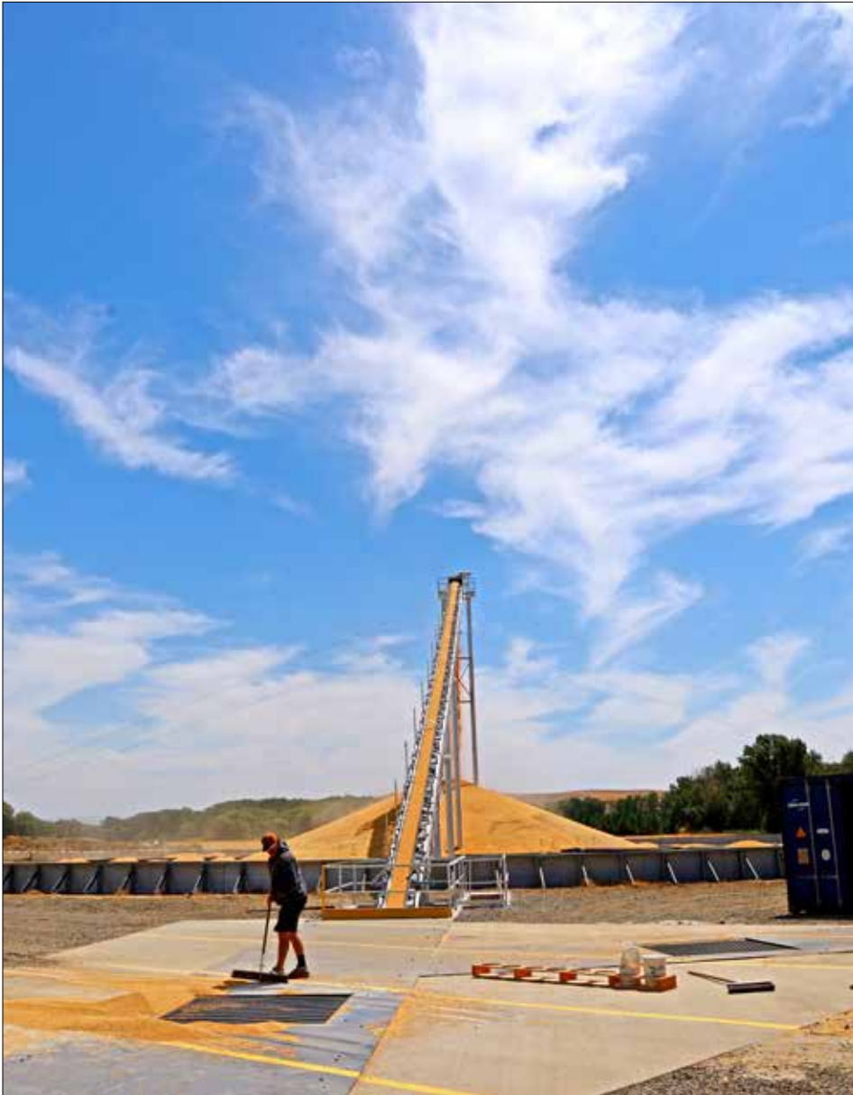
One of Prescott's two ground pile storage units. Grain is emptied into the pit from a truck, taken to the top by the leg system, the same as other elevators. When the pile is complete it is covered by tarps.
